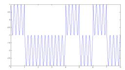
Fig. 6 Amplitude Modulated wave with first input signal.
