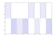
Fig. 7 The output from BASK block Frequency modulated using the second input.
