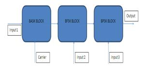
Fig.1 Transmitter Block Diagram
